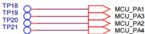
Testpoint TP19, TP20 and TP18 is located next to UART1 (covered when the Som is assembled)
