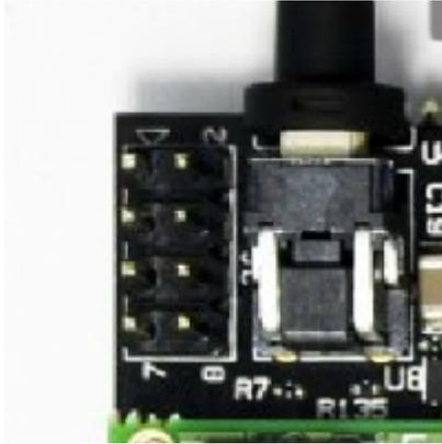
For flashing the bios via the headers, you can use tools like [DediProg SF600Plus](#) and connect it to the Header of the SolidPC Carrierboard.
